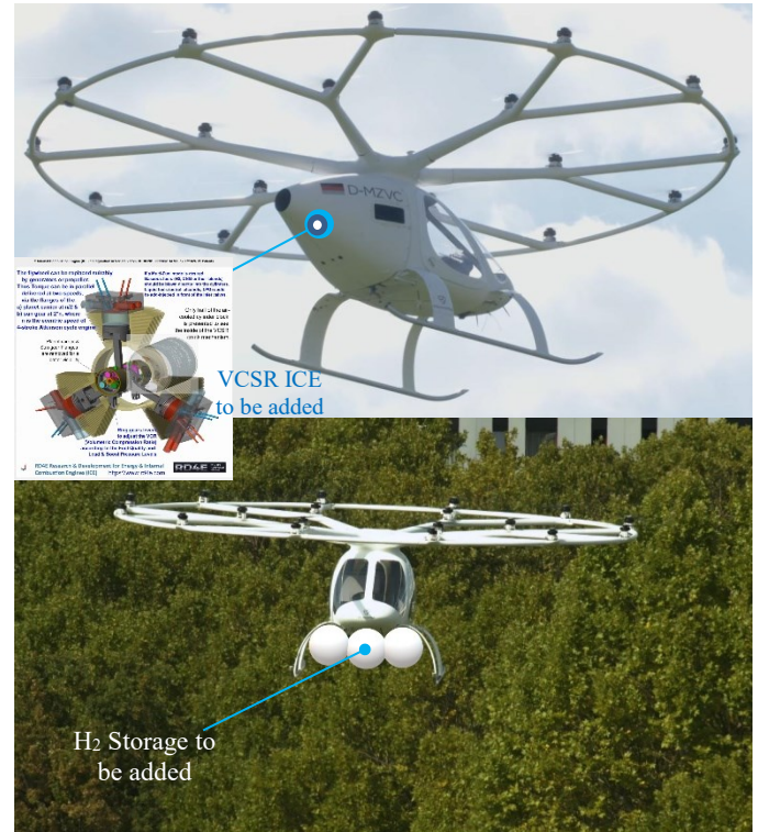
Figure 7-2. Proposed new Design of Volocopter, Volocity Flight-Taxi.
