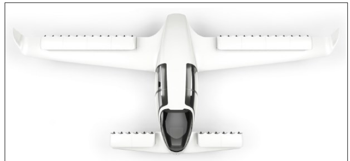
Figure 7-6. Lilium Jet five-seater geometry.
