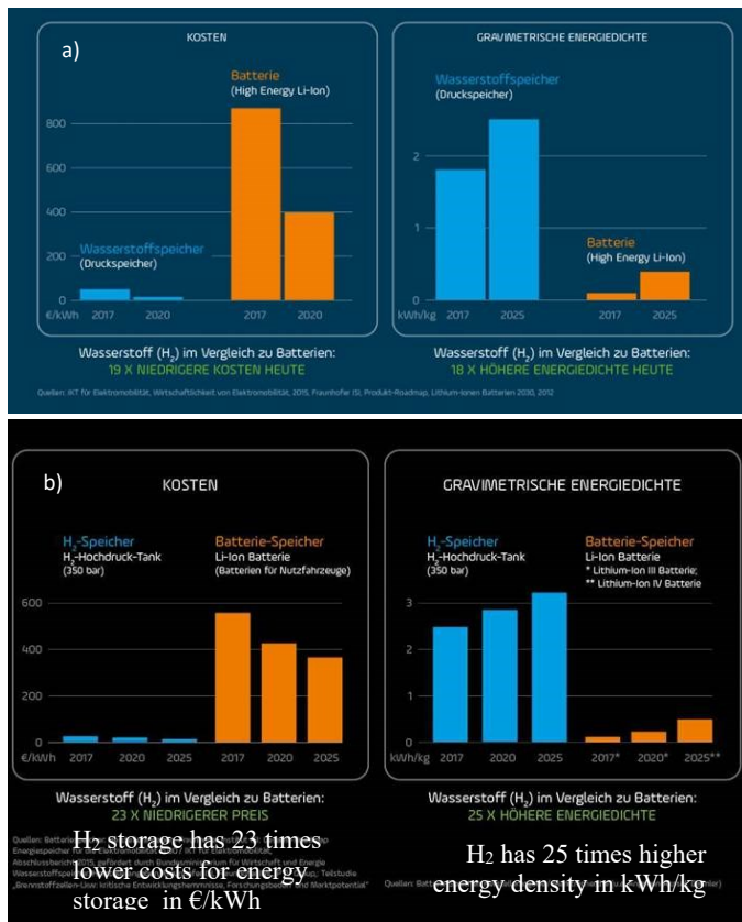
Figures 4-1. ISI Reports, a) 2012 and b) 2015. Costs on the left side versus gravimetric energy density on the right side. Orange are the values for the batteries and the blue ones for H 2 storages, Source ISI. Additional information
